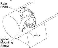
Figure 18 - Removing Ignitor Mounting Screw and Ignitor
